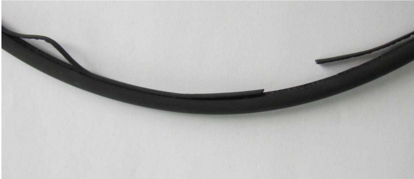
Damage to the O-ring caused by sharp-edged components.
