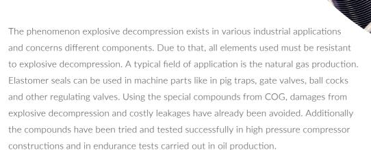
All compounds ensure a long-time sealing performance even if an extremely sudden change in pressure takes place. Next to a high chemical and thermal resistance the compounds offer a hardness which counteract a possible gap extrusion and avoid explosive decompression.
